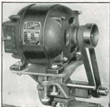
View of 10-450 heavy-duty grinder with belt guard removed, showing two-step pulleys, built-in switch, and belt-tensioning screws.
