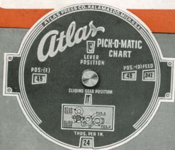
EXAMPLE OF WORK RANGE OF PICK-O-MATIC CHANGE GEARS Selected Instantly Without Changing Gear Train
